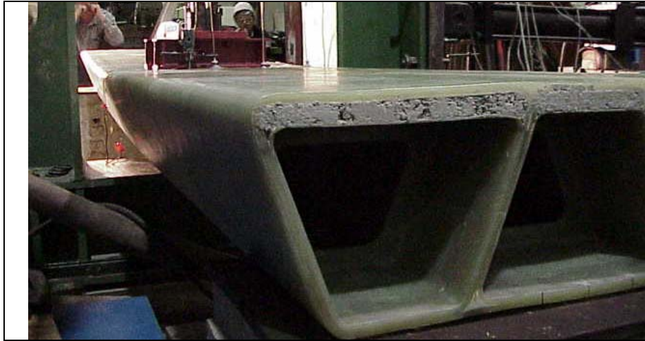
Figure 14. Hybrid deck developed for New York State DOT at University at Buffalo
